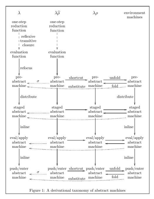
Reading down each column follows Danvy and Nielsen's work on refocusing [20]. They show how to go from a reduction-based evaluation function (obtained as the reflexive-transitive closure of a one-step reduction function) to a pre-abstract machine, and then to a staged machine, an eval/apply machine, and, for call by name and right-to-left call by value, a push/enter machine.
